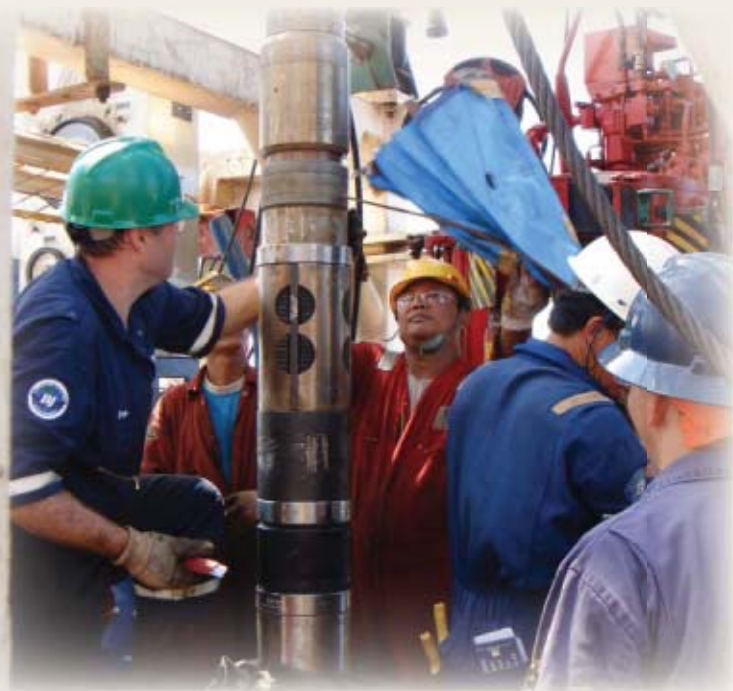
BJ Services' ComPLETE™ MST (multizone, single-trip) system is shown being deployed in a well in Indonesia. The downhole tool system facilitates single-trip gravel- or frac-packed completions across multiple production intervals. Photo courtesy of BJ Services.
